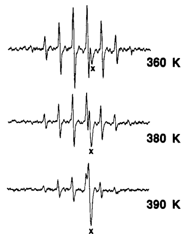
Figure 3. ESR spectra of (CH 3 ) 3 COC 60 • obtained by photolysis of di- tert -butyl peroxide in tert -butylbenzene saturated with C 60 showing the growth of the methyl radical adduct (marked with an X) as the temperature increases.
